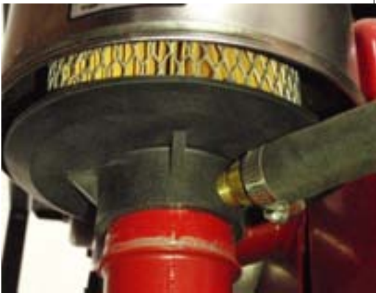
Figure 18. Venturi mixer/air cleaner base installed above the gasoline carburetor. Either fuel may be used, but not both at the same time.
