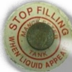
Figure 89. 80 percent fixed maximum liquid level gauge
