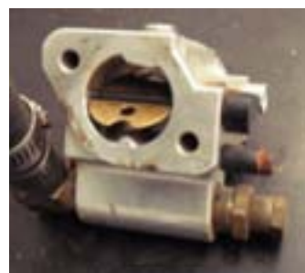
Figure 39. Single-bore mixer for a single-cylinder engine
