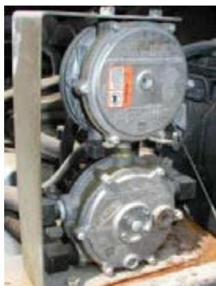
Figures 60 and 61. Approximate location of the vaporizer and lockoff assembly and the vaporizer.
