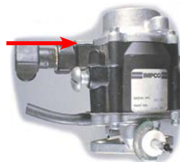
Figure 66. Series 55 max gas flow adjustment
