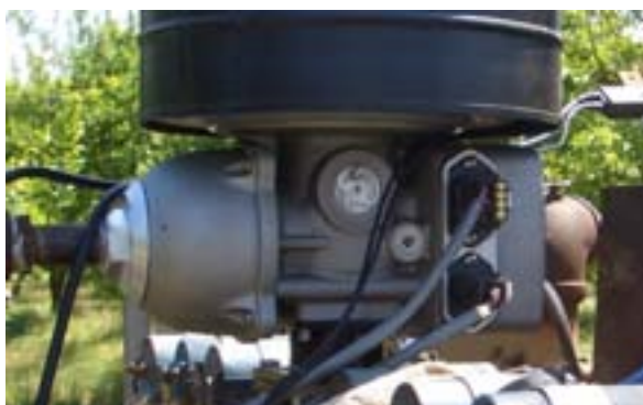
Figure 44. Continental Controls fixed venturi with electronic controls
