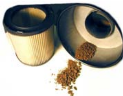
Figure 57. Dirt in air-filter assembly
