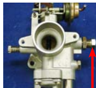
Figure 68. Aisan max gas flow adjustment
