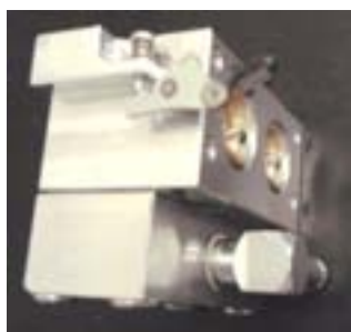
Figure 38. Dual-bore mixer for a V-twin engine
