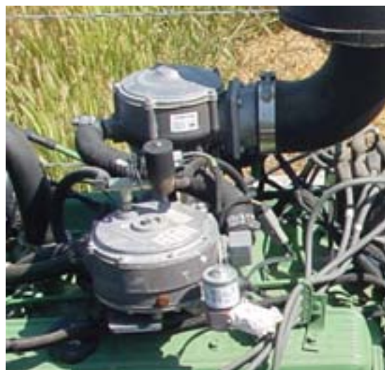
Figure 19. Liquid fuel system with electronic controls
