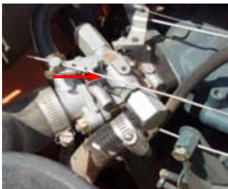
Figure 40. Mixer for Kubota 3-cylinder engine
