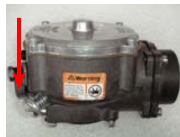
Figure 67. Series 100-125-200-225 max gas flow adjustment
