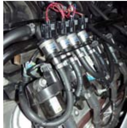
Figure 27. Vapor phase fuel injectors mounted on a General Motors 6.0 engine
