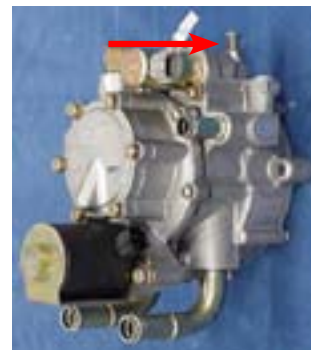
Figure 65. Idle mixture adjustment on Aisan vaporizer
