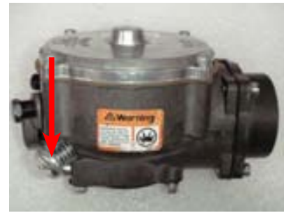
Figure 63. Idle mixture adjustment screw on Series 100 mixer
