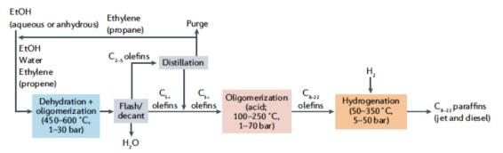
Figure 17. Three step process for producing hydrocarbons from ethanol.<sup>37</sup>
