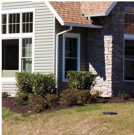
Propane storage can be buried underground with only an inconspicuous service dome showing.
