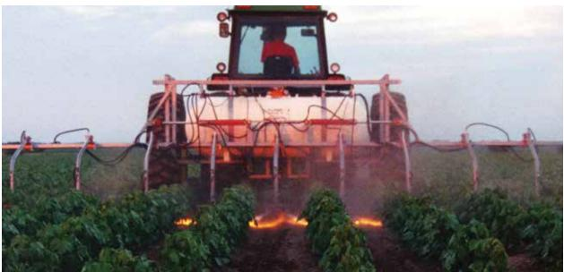
A steam/flame weed control system is used in fields with a tractor mount for large crop sites.
