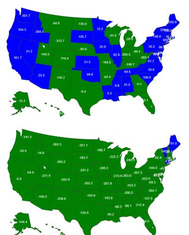
**Figure 4**: CO2eq emissions comparisons between a propane and an electric school bus using baseload (above) and non-baseload (below) emissions.
