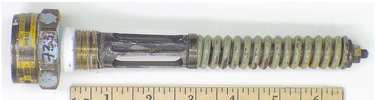
Figure 122. PRV 733, 275-psig Set Pressure PRV that Exhibited Low STD Behavior. This PRV was 50 years old.
