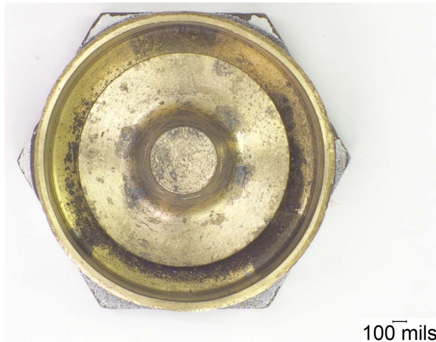
Figure 85. Slight Discoloration of the Inside Surface of the Housing and the Gasket Holder from PRV 674.
