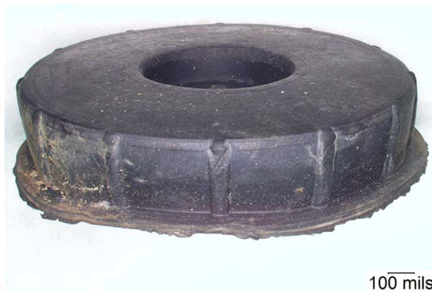
Figure 65. Ribs on the Surface of the Internal Rain Cap from PRV 116. According to experienced personnel, even rain caps that remain in place on the PRV can curl up and allow rain to enter the PRV housing.
