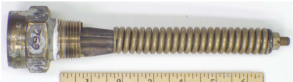
Figure 108. PRV 696, 250-psig Set Pressure PRV that Exhibited High STD Behavior. This PRV was 57 years old.
