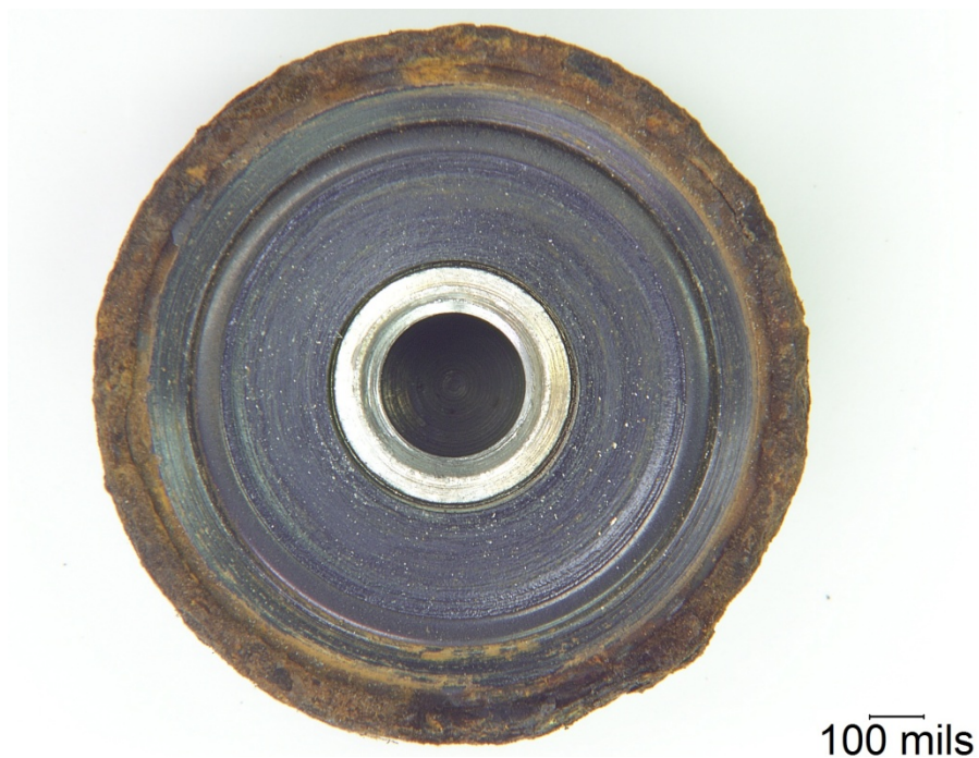
Figure 83. Severely Corroded Bottom Surface on the Gasket Holder from PRV 760.
