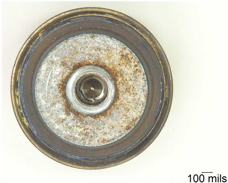
Figure 89. Mixed-Color Corrosion Products on the Surface of the Gasket Washer from PRV 674.
