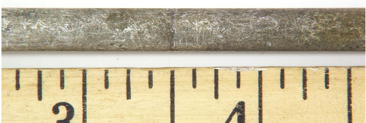
Figure 121. Higher Magnification View of the Surface of the PRV Stem from PRV 597.
