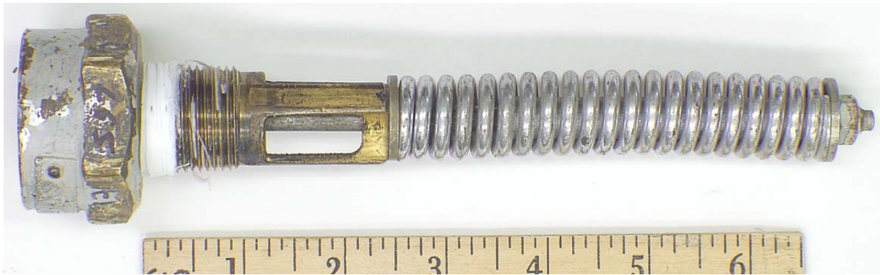
Figure 115. PRV 597, 275-psig Set Pressure PRV that Exhibited Low STD Behavior. This PRV was 40 years old.
