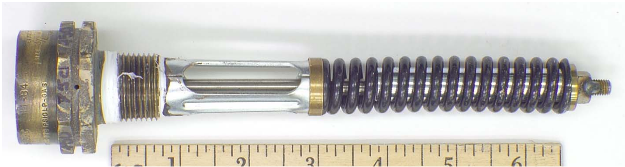
Figure 96. PRV 750, 250-psig Set Point PRV that Exhibited High STD Behavior. This PRV was 27 years old.
