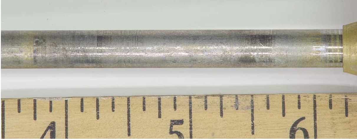
Figure 81. Circumferential Rub Marks on the Surface of the Stem from PRV 760. The rub marks were caused when the stem turned during disassembly.
