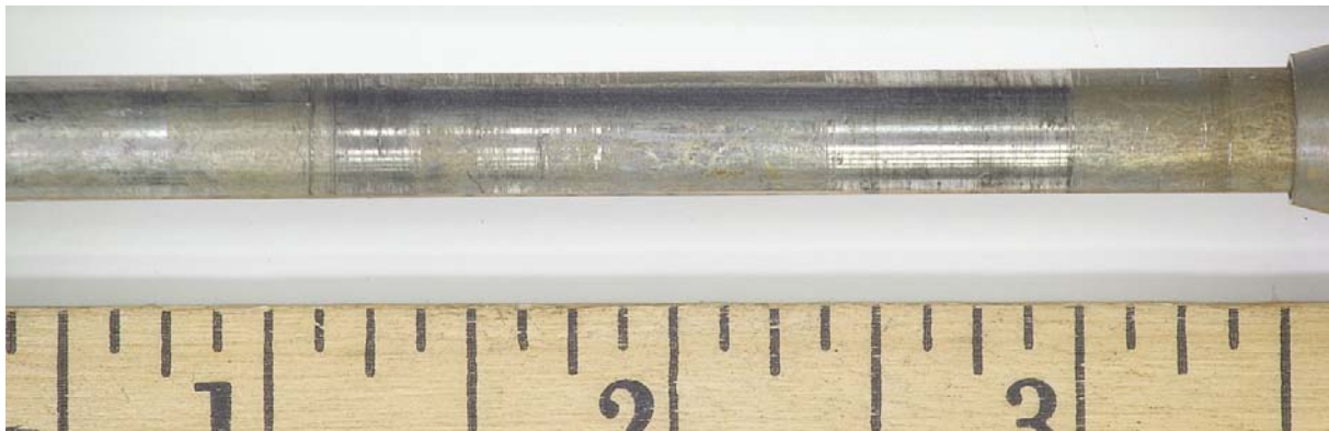
Figure 79. Circumferential Rub Marks on the Surface of the Stem from PRV 122. The rub marks were caused when the stem turned during disassembly.
