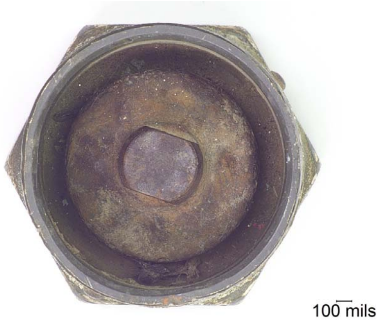
Figure 75. Discoloration of the Inside Surface of the Housing, Debris Inside the Housing, and Rust on the Surface of the Gasket Holder from PRV 122
