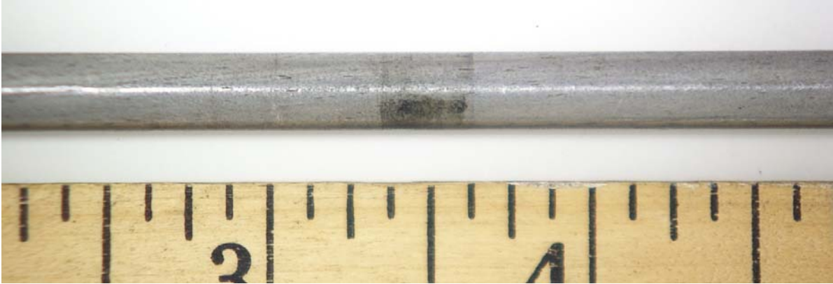
Figure 101. Mark on the Surface Formed by Contact Between the PRV Stem and the Spacer/Guide from PRV 395.
