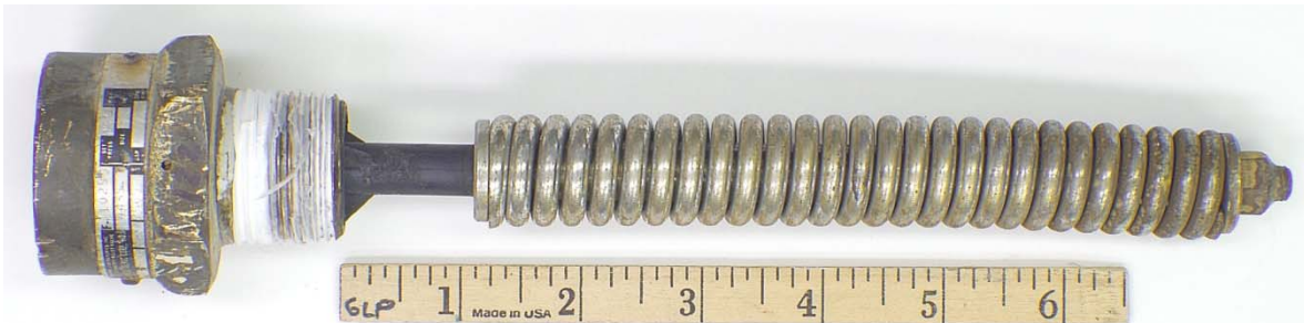
Figure 73. Overall View of PRV 122 (275-psig Set Pressure) that Did Not Open During Pressure Testing. Note the bow in the spring.
