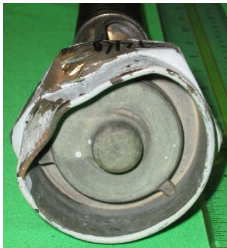
Figure 39. Top View of PRV 746 Showing Significant Physical Damage
