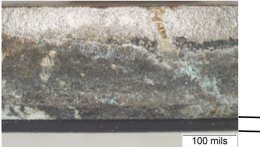
Figure 59. Thin Gasket on the Surface of the Gasket Holder from PRV 559. The gasket was about 0.025-inch thick. The black lines indicate the thickness of the gasket.
