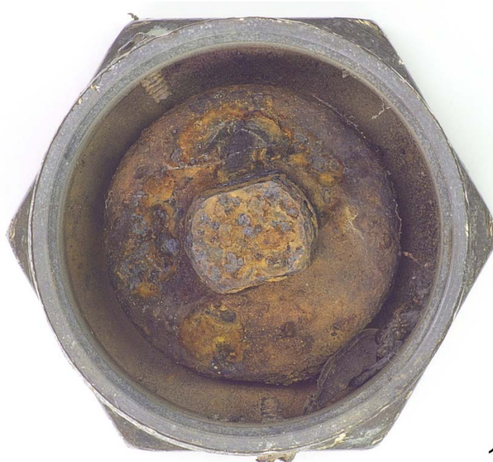
Figure 77. Discoloration of the Internal Surface of the Housing, Debris Inside the Housing, and Rust on the Surface of the Gasket Holder from PRV 760.
