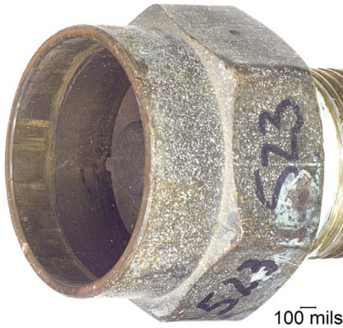
Figure 68. Internal Marks and Rain-Cap Line on the Internal Surface of the Housing from PRV 523.
