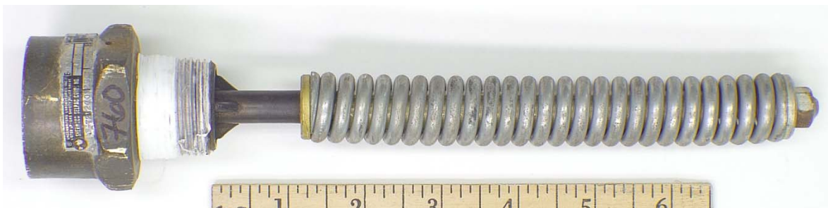
Figure 74. Overall View of PRV 760 (275-psig Set Pressure) that Did Not Open During Pressure Testing. Note the slight bow in the spring.
