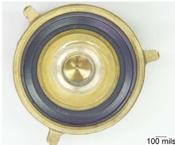
Figure 52. Nonconcentric Compression Set Rings in the Gasket from PRV 116.
