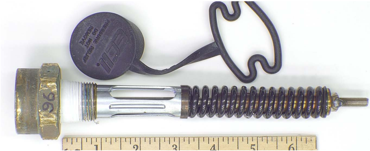
Figure 90. PRV 96, 250-psig Set Pressure, that Exhibited High STD Behavior. This PRV was four years old.
