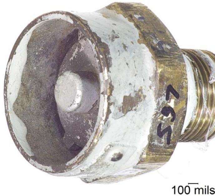
Figure 71. Housing from PRV 597 Showing no Evidence of Internal or External Rain-Cap Lines.
