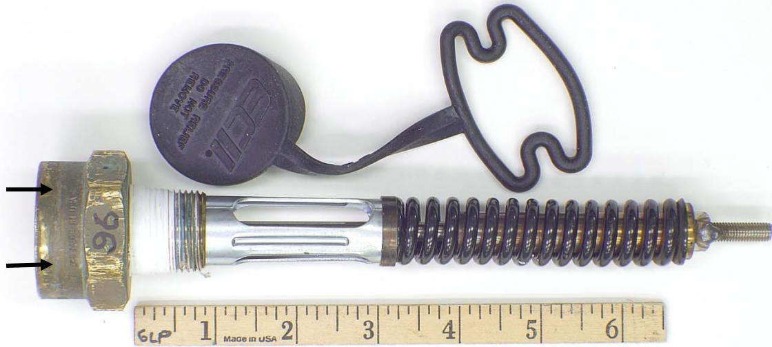
Figure 63. PRV 96 with External Rain Cap. Note the faint rain-cap line (arrows) on the surface of the housing.
