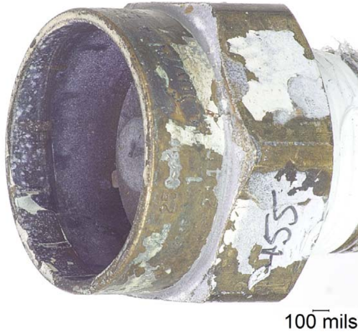
Figure 67. Marks on the Inside Surface of the Housing from PRV 455 Indicating that an Internal Rain Cap had been Present for Only a Portion of the Service Life of the PRV.
