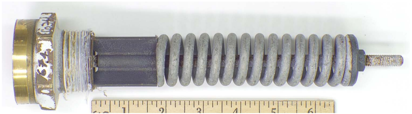
Figure 84. Overall View of PRV 674, 250-psig Set Pressure PRV that Exhibited High STD Behavior.
