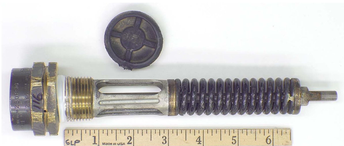
Figure 64. PRV 116 with an Internal Rain Cap.
