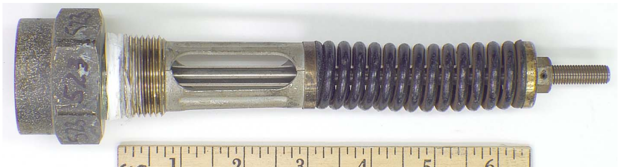
Figure 102. PRV 523, 275-psig Set Pressure PRV that Exhibited High STD Behavior. This PRV was 31 years old.
