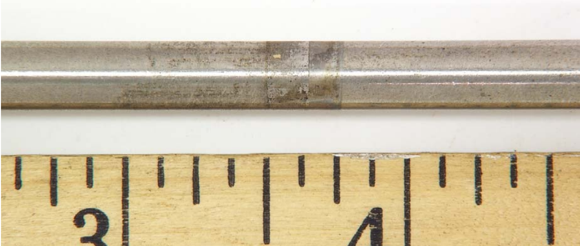
Figure 98. Mark on the Surface Formed by Contact Between the PRV Stem and the Guide Washer from PRV 750.
