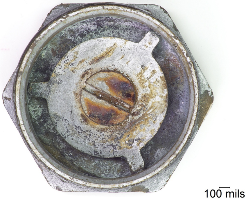
Figure 47. Slotted head on the Stem from PRV 559
