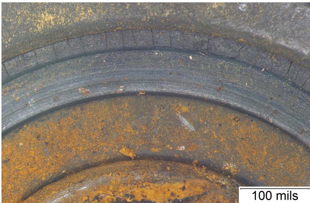
Figure 114. Rust Deposits on the Surface of the Gasket and the Gasket Washer that were Exposed to a Propane Environment During Service and Rust Particles on the Seal Region Surface.
