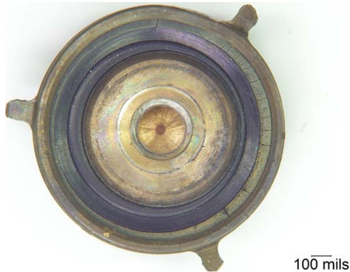
Figure 53. Nonconcentric Compression Set Rings and Multiple Radial Cracks in the Outer Circumferential Ring of the Gasket from PRV 174.
