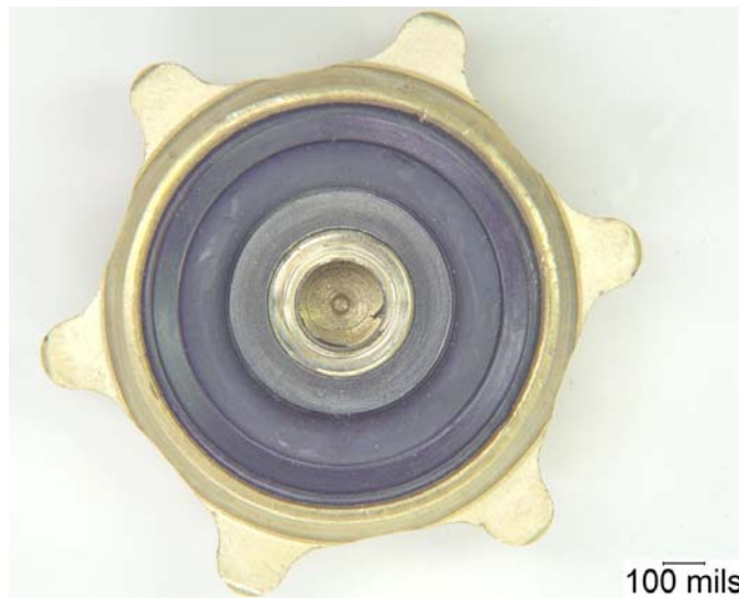
Figure 51. Concentric Compression Set Rings in the Gasket from PRV 96.
