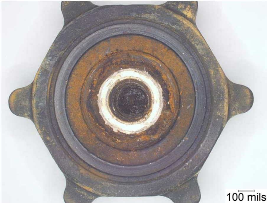
Figure 113. Rust Deposits on the Surface Region of the Gasket that was Exposed to a Propane Environment During Service.
