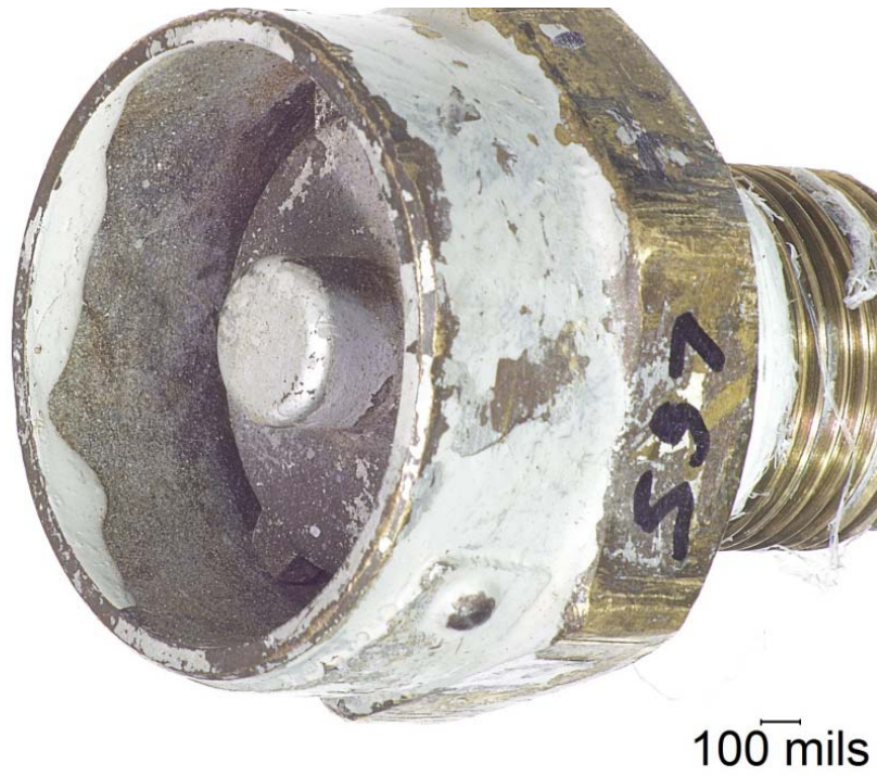
Figure 116. Discoloration and Paint on the Internal and External Surfaces of the Housing from PRV 597.
