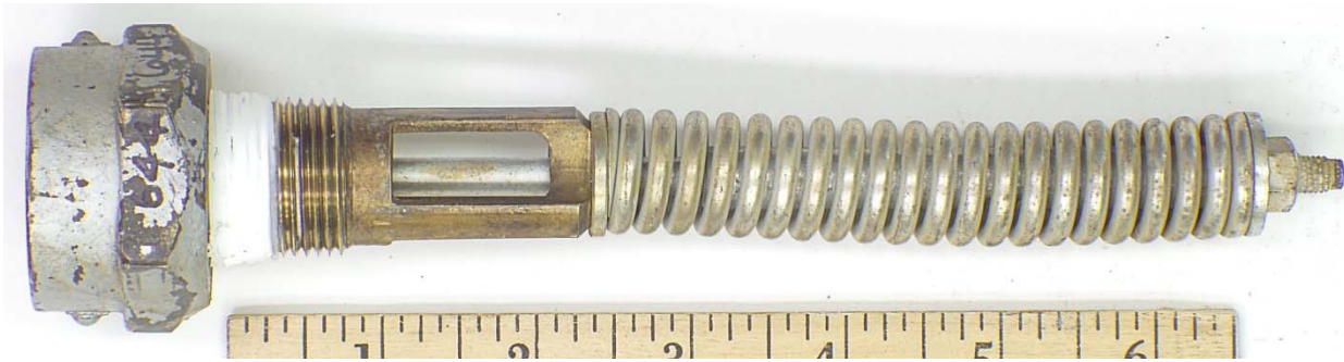
Figure 105. PRV 644, 250-psig Set Pressure PRV that Exhibited High STD Behavior. This PRV was 53 years old. Note the bow in the spring.
