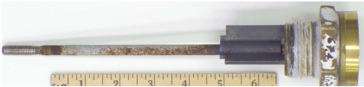
Figure 88. Mixed-Color Corrosion Products on the Surface of the Stem from PRV 674.
