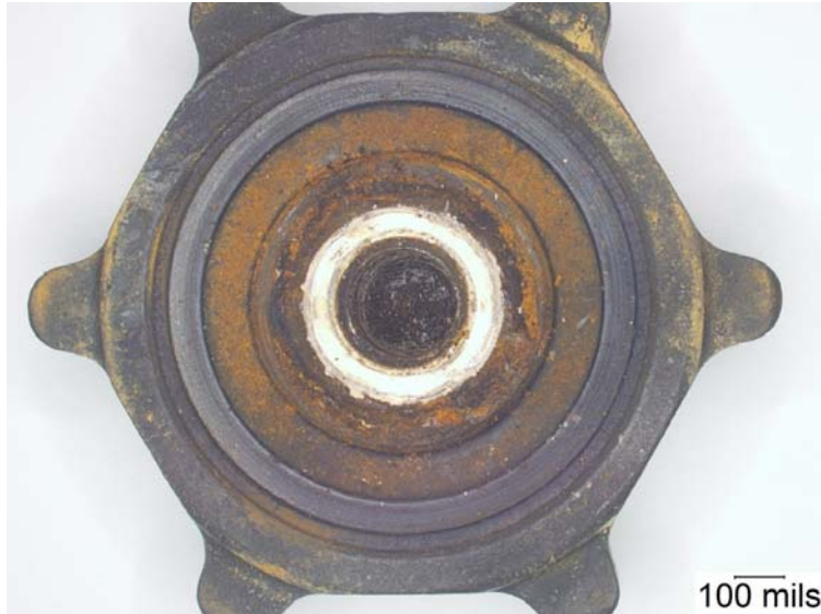
Figure 61. Rust on the Surface of the Gasket and the Washer from PRV 187. The rust was on the portion of the surface that was exposed to propane.
