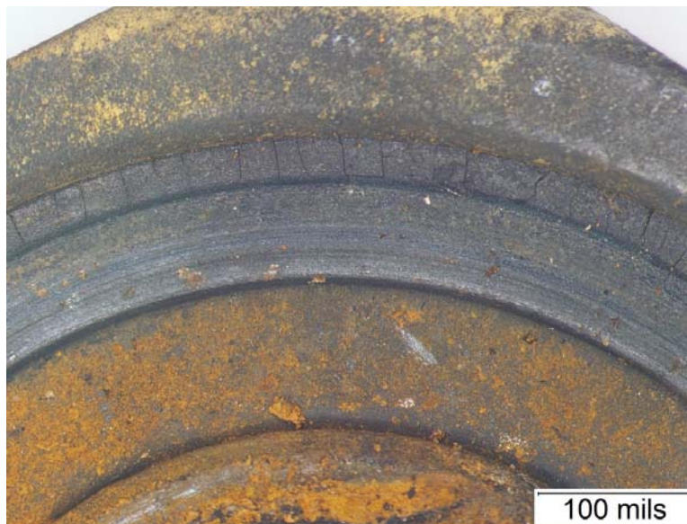
Figure 62. Higher Magnification View Showing Rust Particles on the Seal Portion of the Surface of the Gasket from PRV 187. Note also the radial cracks in the outer ring of the gasket.
