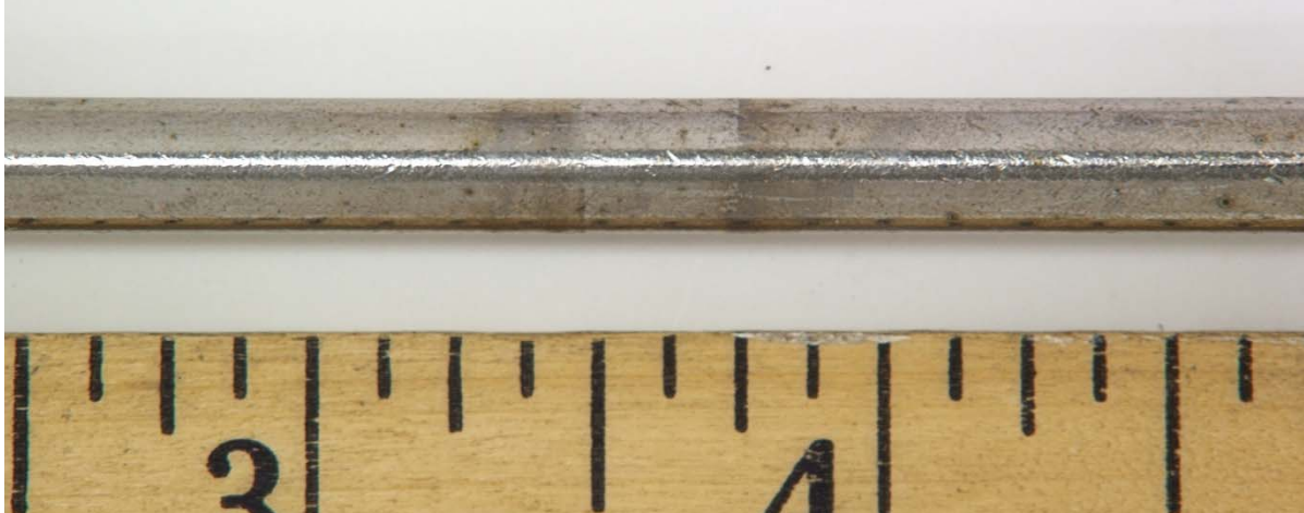
Figure 92. Mark on the Stem Formed by Contact between the PRV Stem and the Guide Spacer/Washer from PRV 96.
