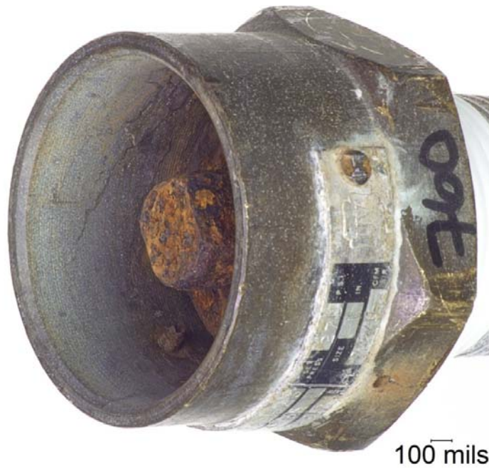
Figure 72. Housing from PRV 760 Showing no Evidence of Internal or External Rain-Cap Lines.
