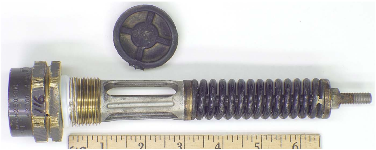
Figure 93. PRV 116, 250-psig Set Pressure PRV that Exhibited High STD Behavior. This PRV was 16 years old.
