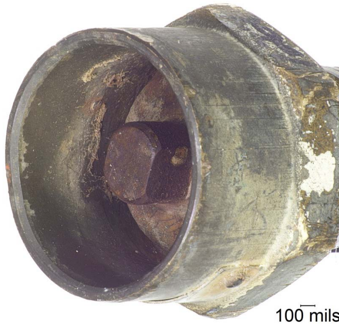
Figure 76. Additional Debris on the Inside Surface and the Absence of Rain-Cap Lines on the Internal and External Surfaces of the Housing from PRV 122.
