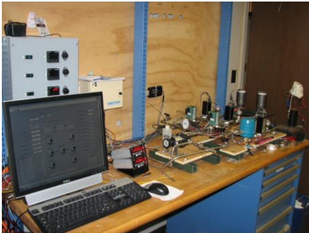
Figure 23. Start-to-Discharge Test Stand
