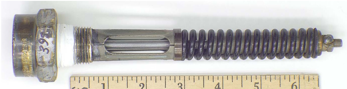
Figure 99. PRV 395, 250-psig Set Pressure PRV that Exhibited High STD Behavior. This PRV was 31 years old.
