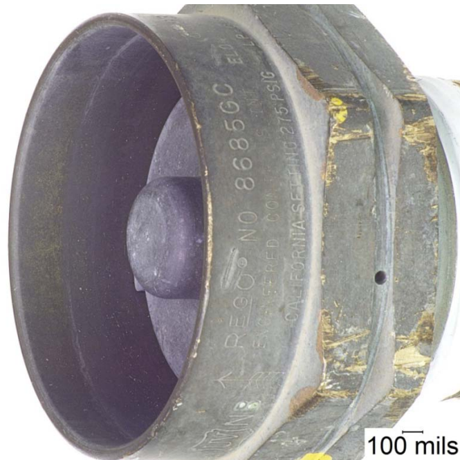
Figure 69. Faint Internal Rain-Cap Line on the Housing from PRV 140.
