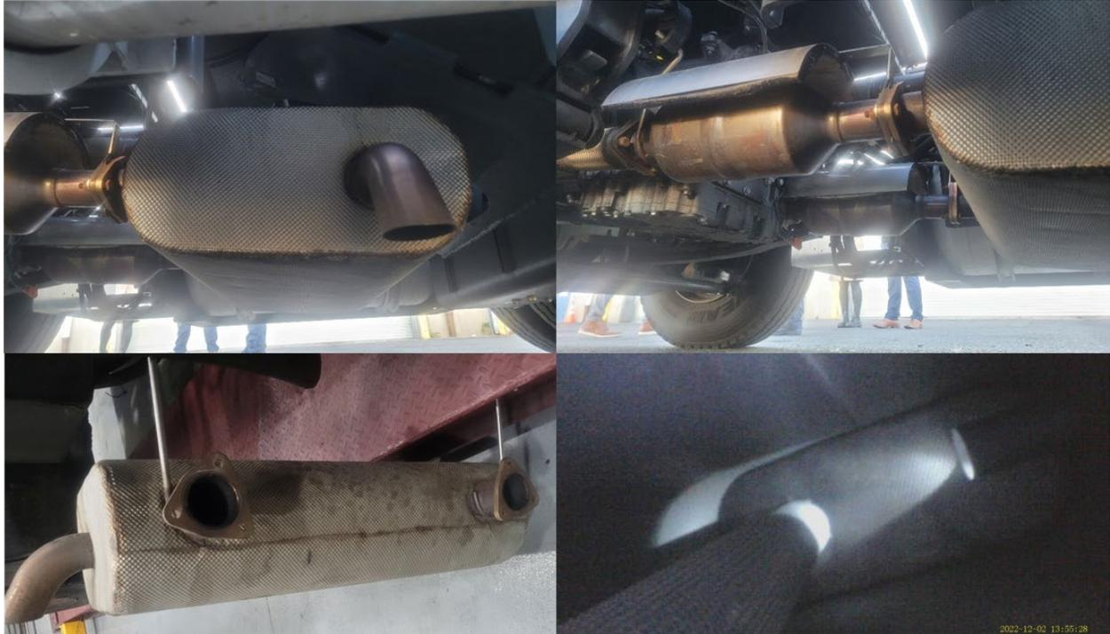
**Figure 8.3 Exhaust System Components of MAFI Port Tractor H1**
