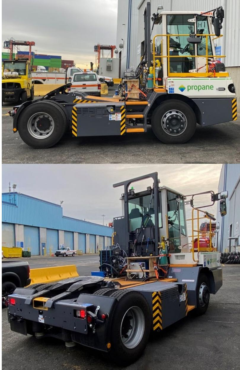
**Figure 8.2 PEMS Installation on MAFI Propane-Fueled Port Tractor H1**
