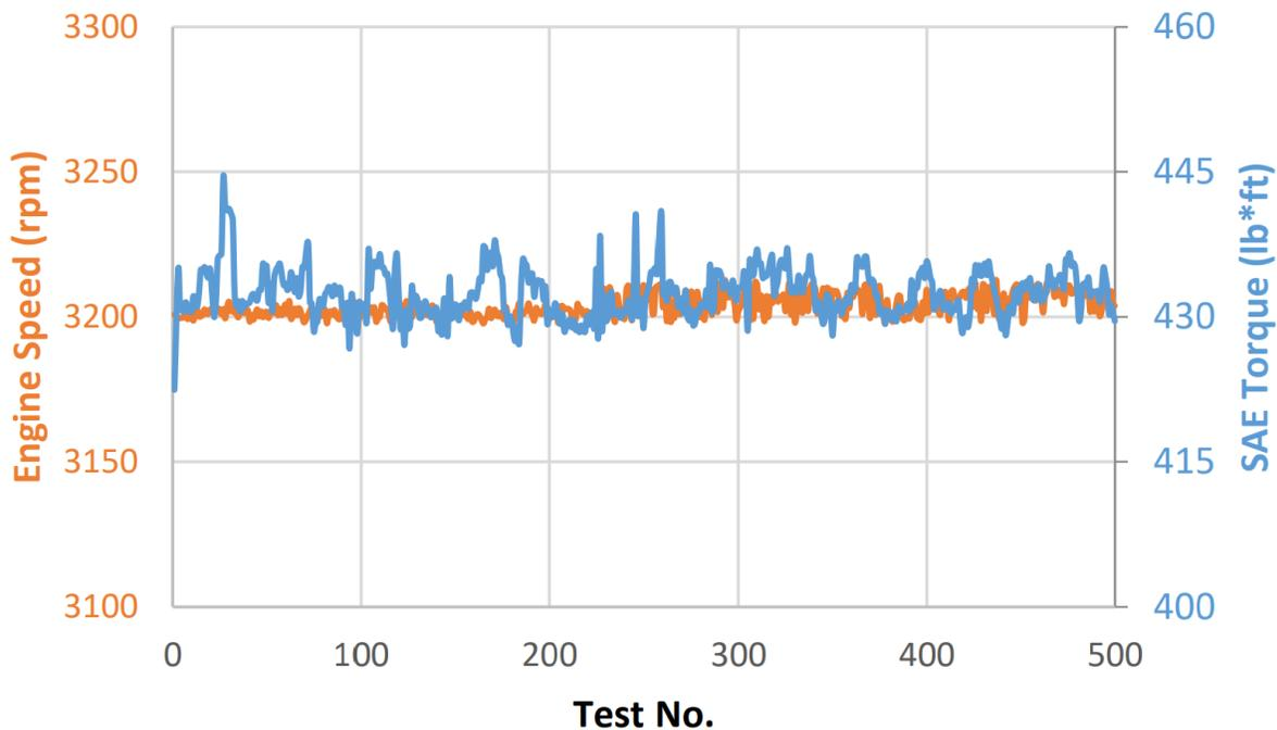
Figure 38: Variation in the engine speed and SAE torque at 3200 RPM WOT during the 250 hrs. durability testing.
