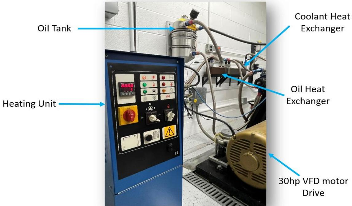
Figure 5: 12 kW heating unit for regulating fuel temperature.
