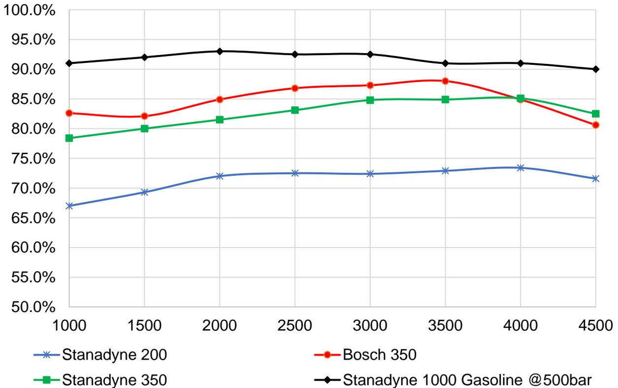
Figure 15: Volumetric efficiency of three DI pumps @100 bar at 30°C fuel temperature compared against volumetric efficiency of gasoline at 500 bar.
