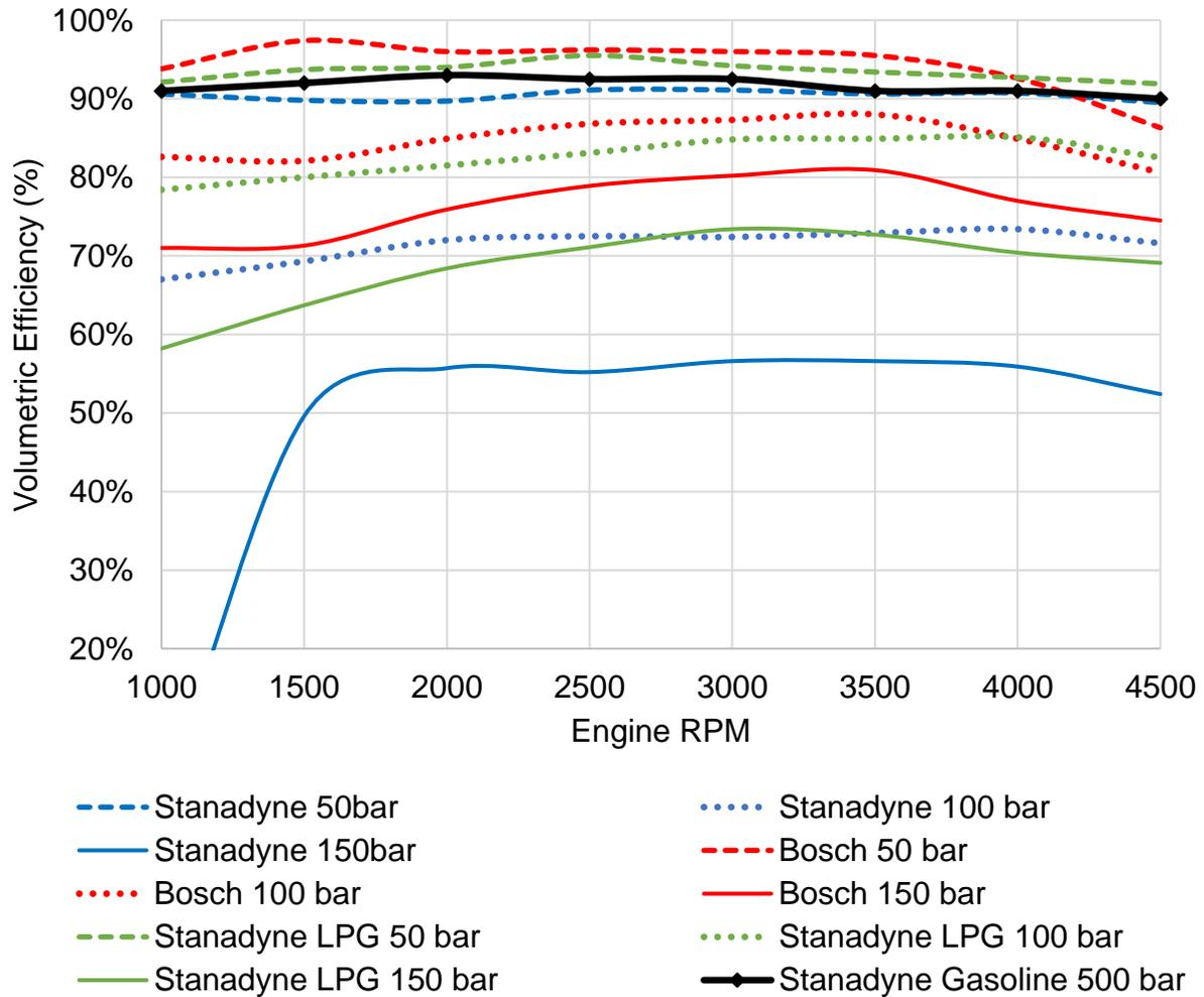
Figure 22: Volumetric efficiency of three DI pumps @50 bar, 100 bar, and 150 bars at 30°C fuel temperature.
