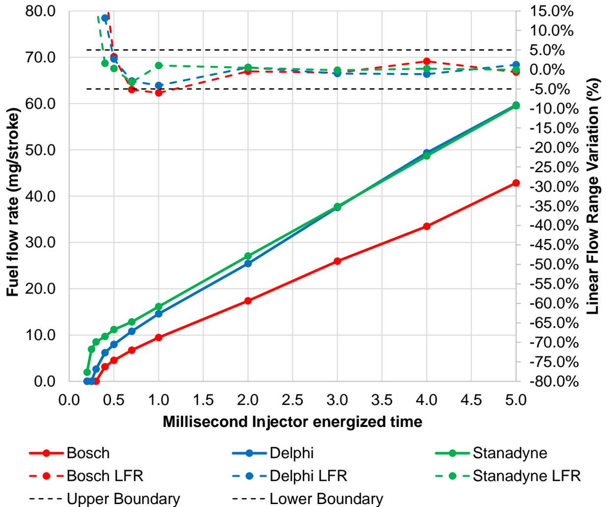
Figure 27: Variation in injection flow rate with respect to pulse width at 100 bar rail pressure
