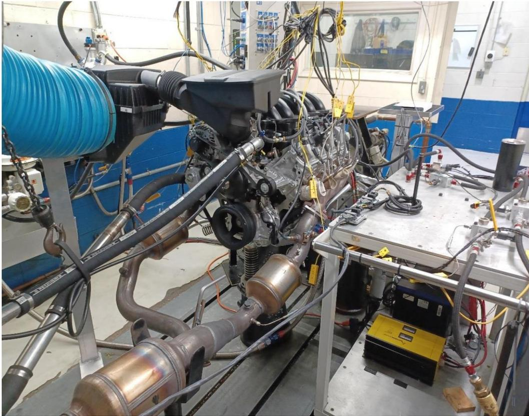
Figure 9: Experimental setup of GM L8T Engine on Superflow dynamometer
