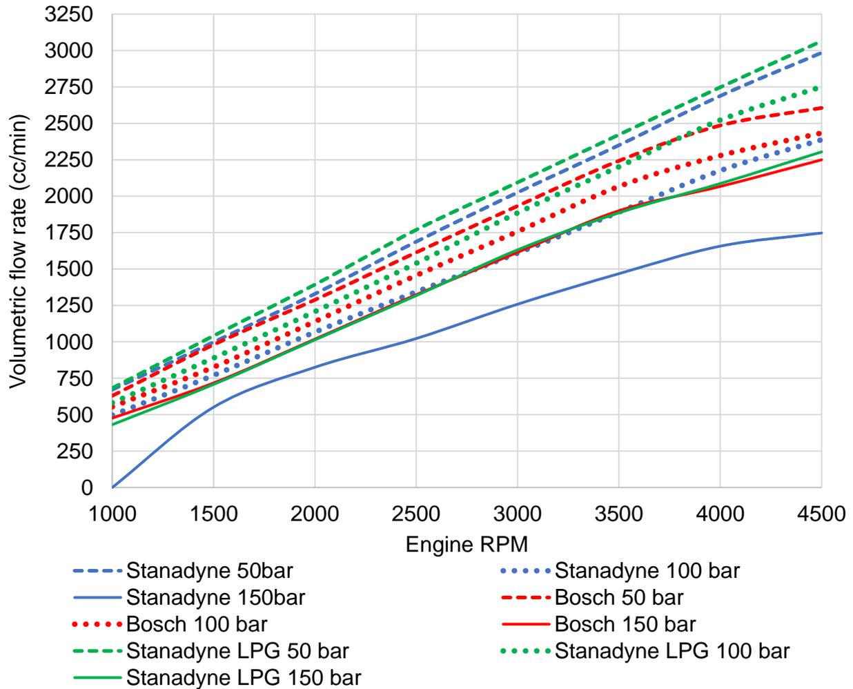
Figure 21: Volumetric flow rate of three DI pumps @ 50 bar, 100 bar, and 150 bars at 30°C fuel temperature.
