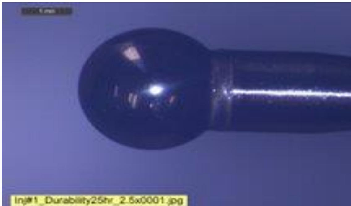
Figure 31: Image of injector needle after 25 hr. injector reliability testing
