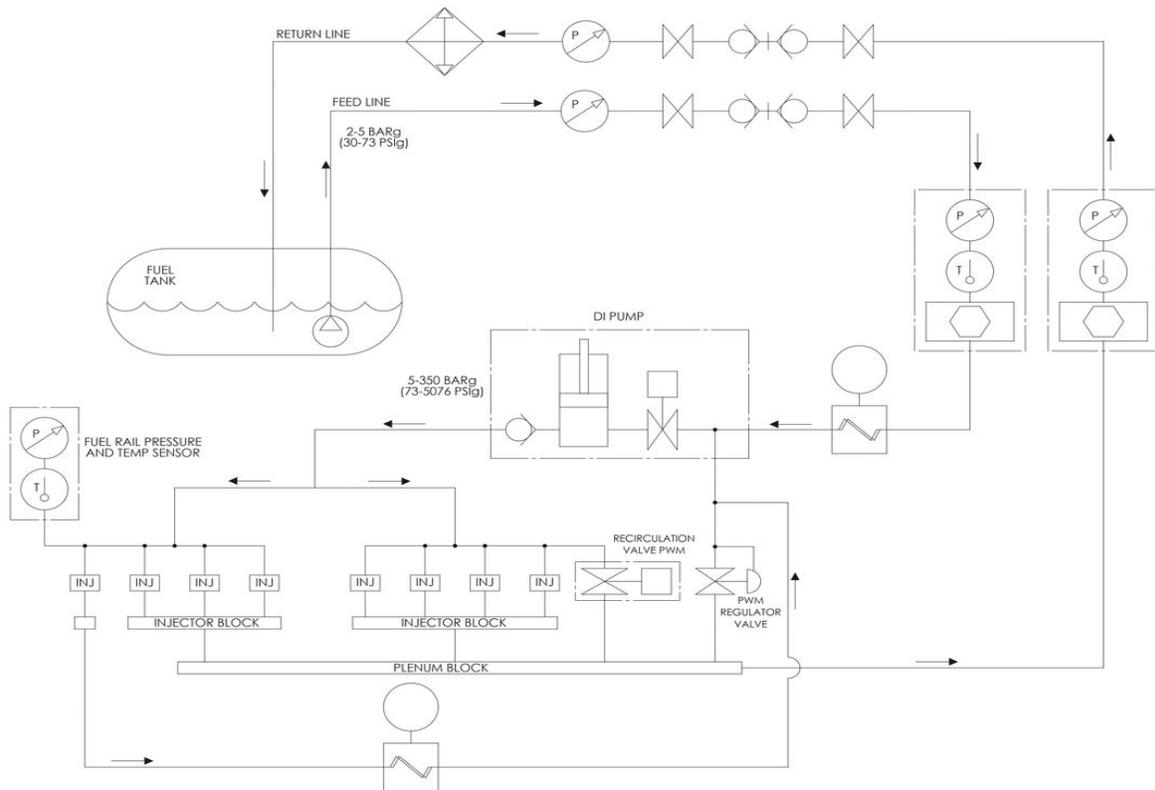
Figure 3: Schematic drawing of the high-pressure DI pump & injector combination test rig
