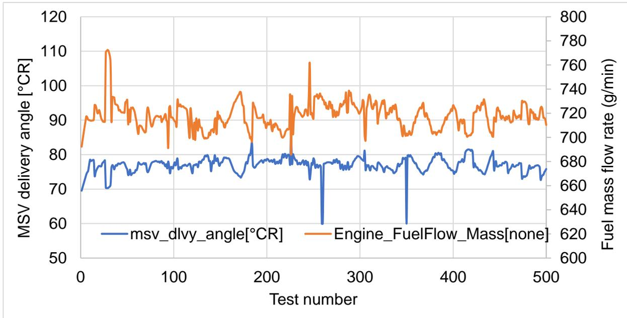
Figure 41: Stable MSV delivery angle and engine fuel mass flow rate of high-side fuel pump during durability testing, 3200 rpm and WOT
