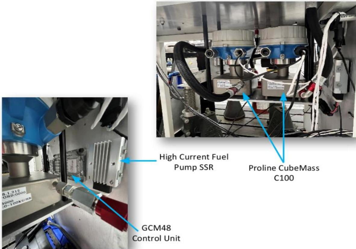
Figure 6: Mass flow meters and control unit used in the proposed test rig
