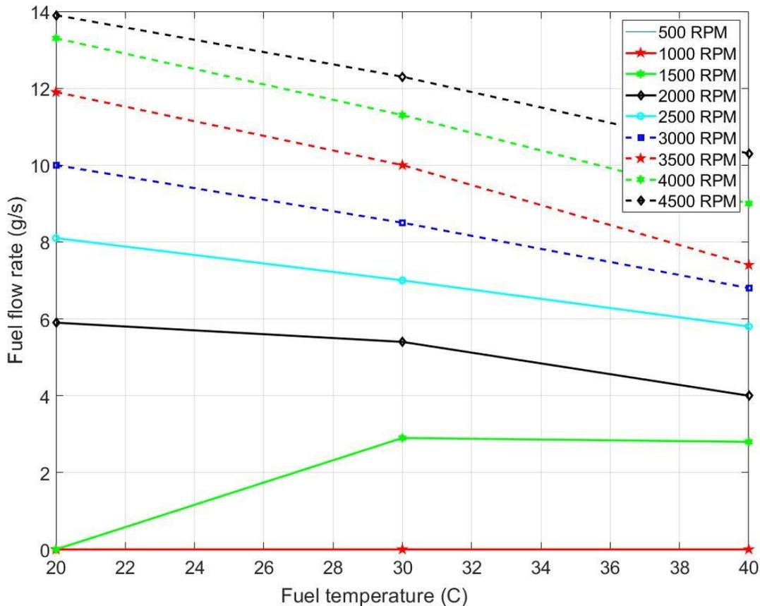
Figure 18: Mass flow rate variations with respect to engine speed and fuel temperature at 175 bar delivery pressure
