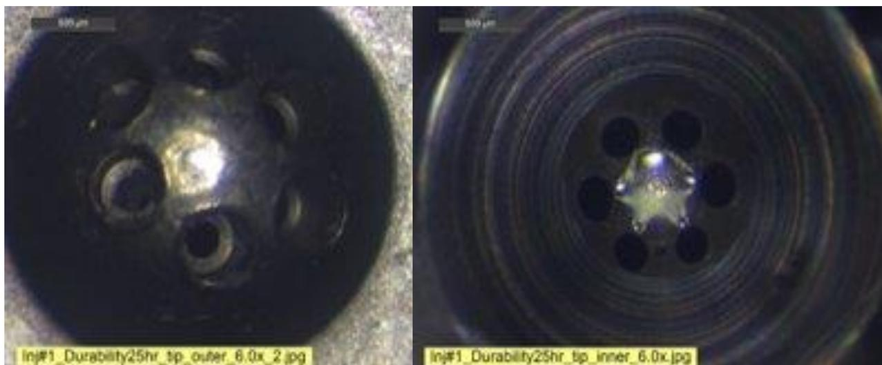
Figure 32: Image of outer and inner injector tips after 25 hr. injector reliability testing
