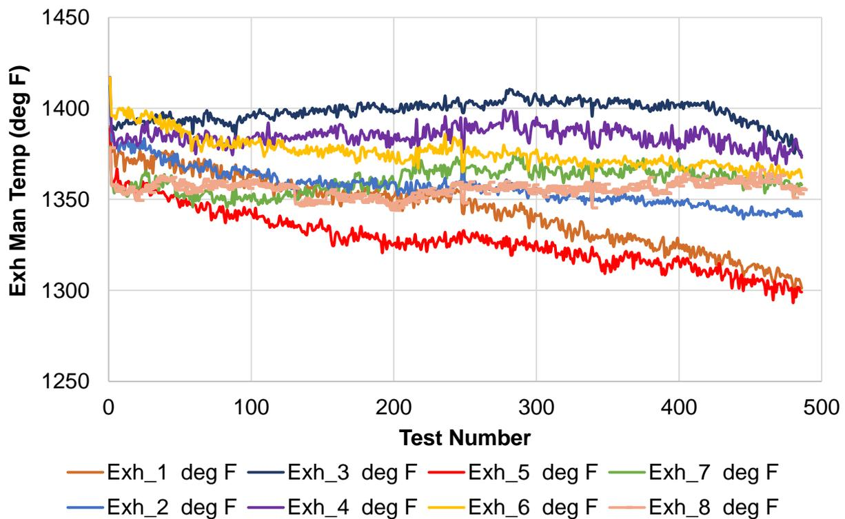
Figure 48: Variation in the cylinder EGTs during durability testing.
