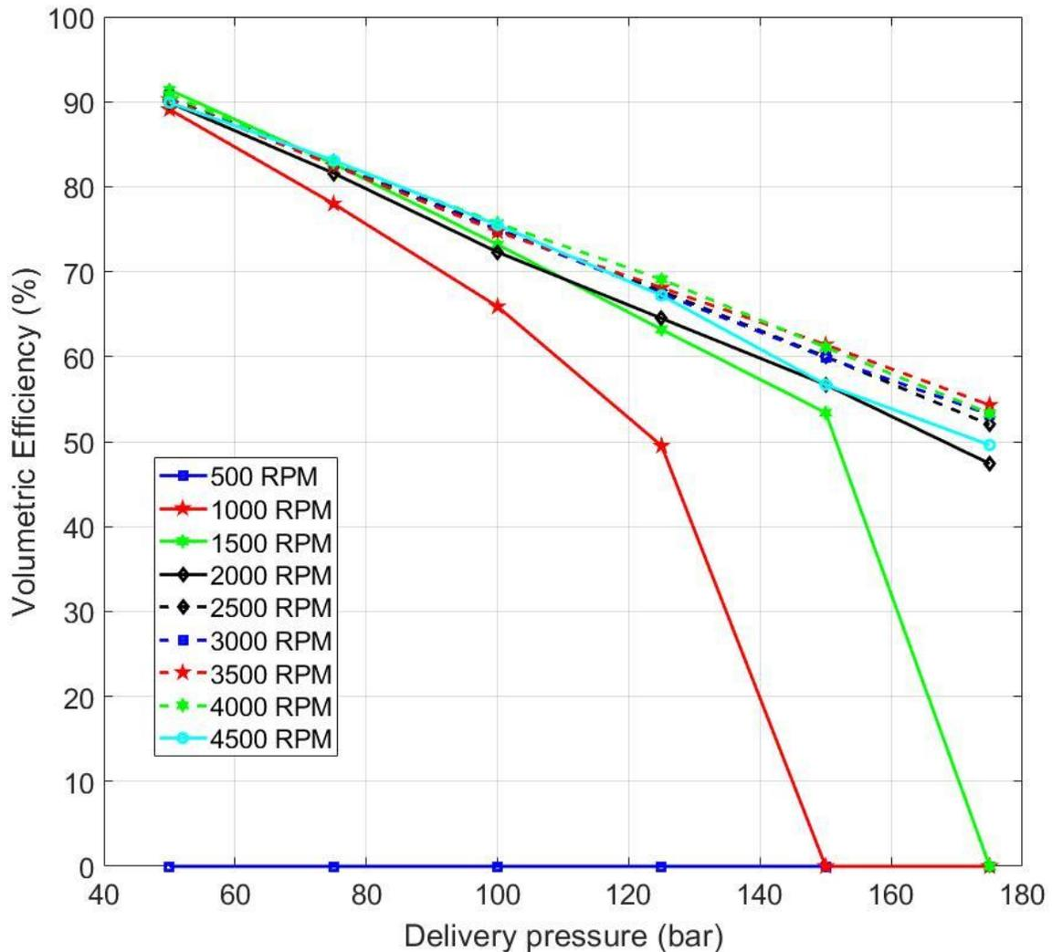
Figure 17: VE variations with respect to engine speed and delivery pressure.
