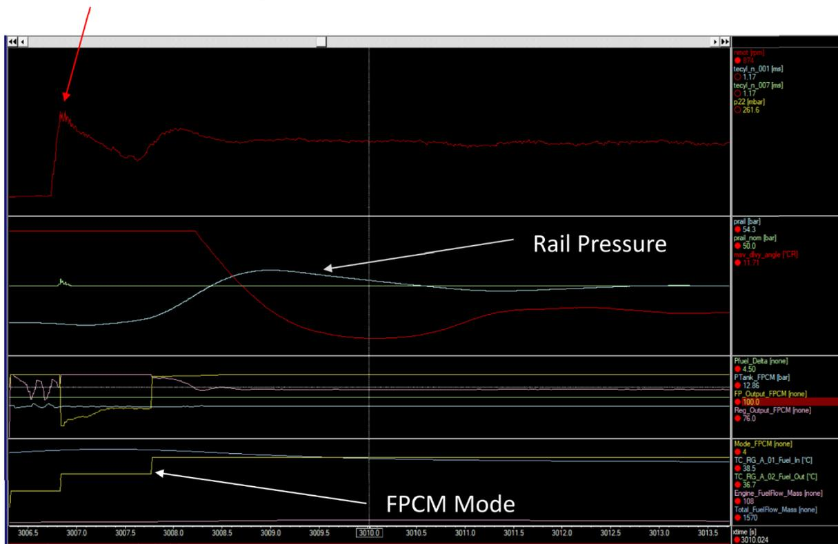
Figure 54: ECU screen depicting the start procedure & mode progression after heat soak.
