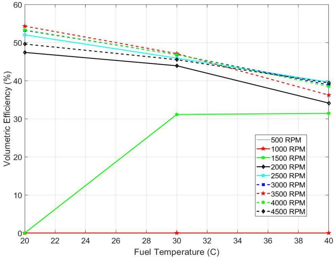
Figure 19: VE variations with respect to engine speed and fuel temperature at a delivery pressure of 175 bar
