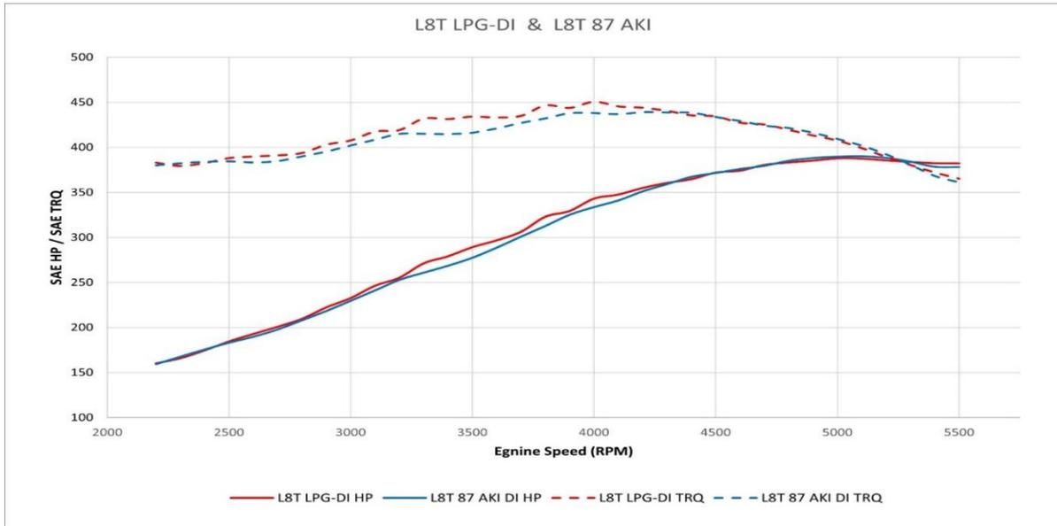
Figure 35: Torque and power characteristics comparison of L8T engine with 87AKI gasoline and LPG DI operation
