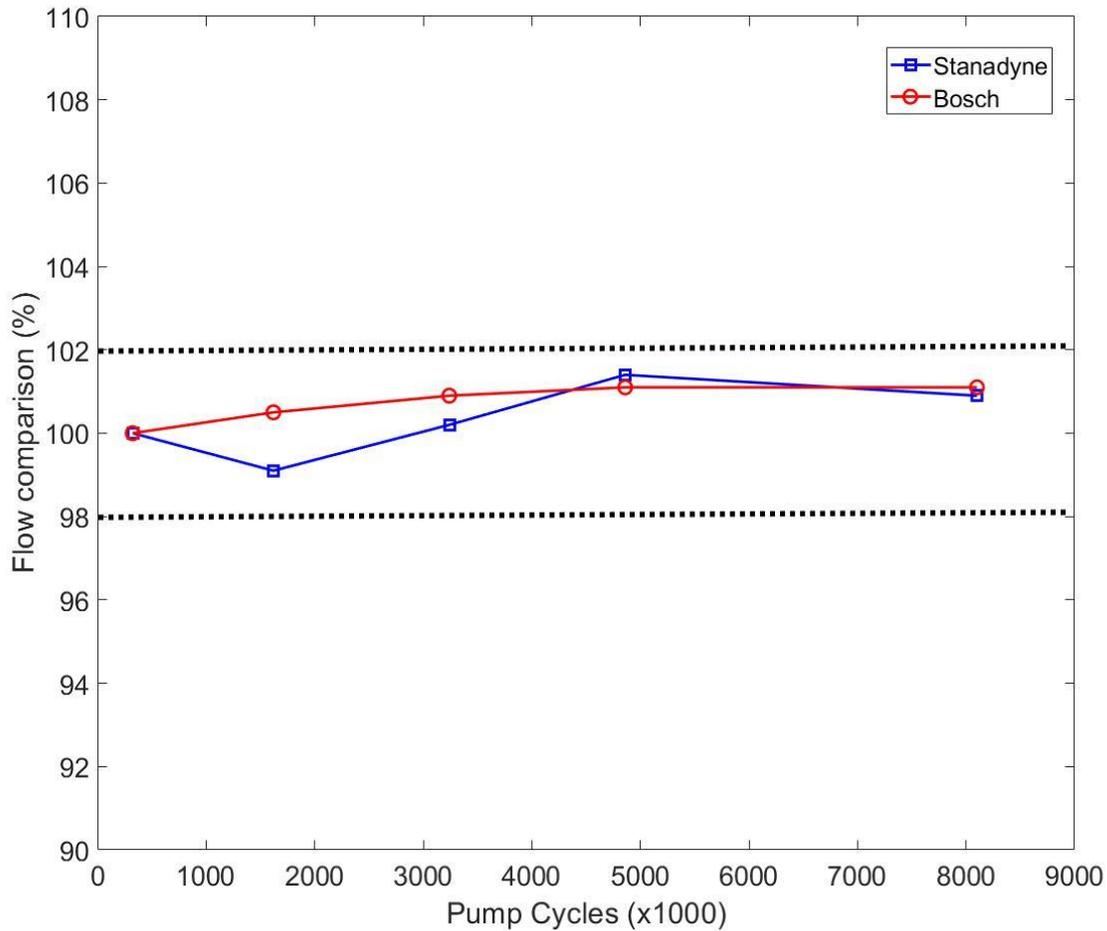
Figure 24: Flow shift variation comparison of Bosch & Stanadyne pumps during limited time durability testing
