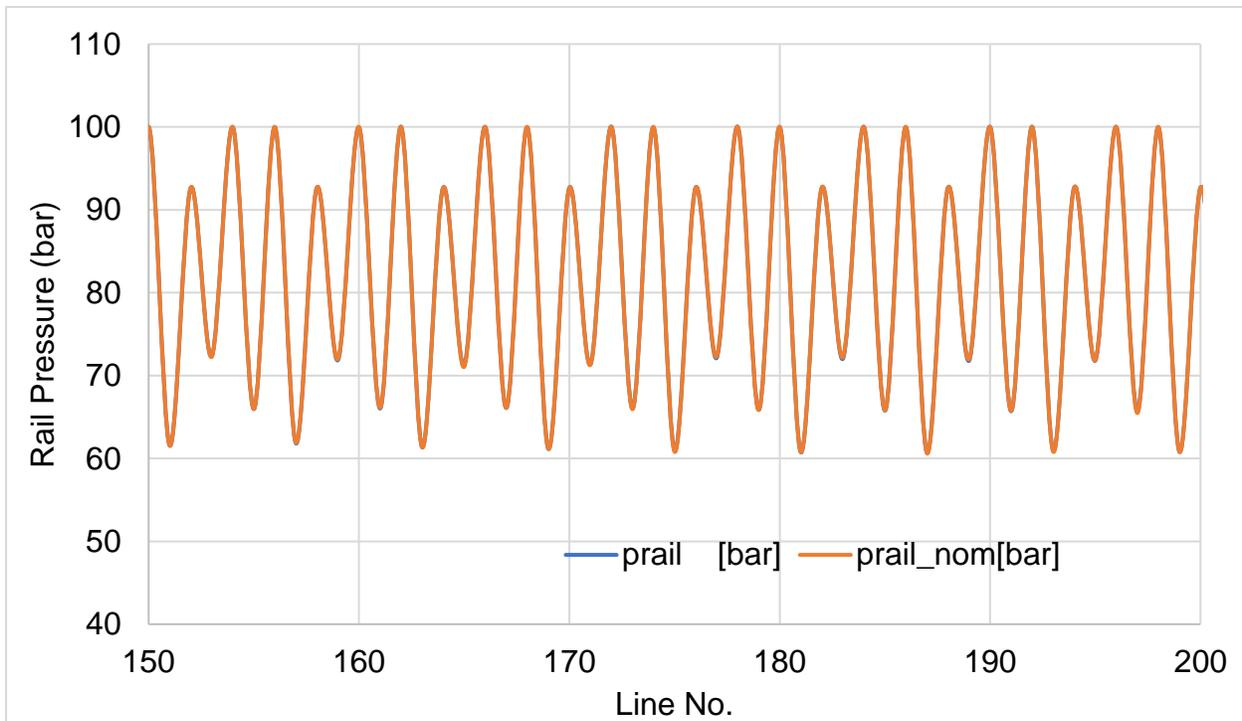
Figure 40: Nominal and actual fuel pressures proving the reliable performance of high-pressure DI pump.
