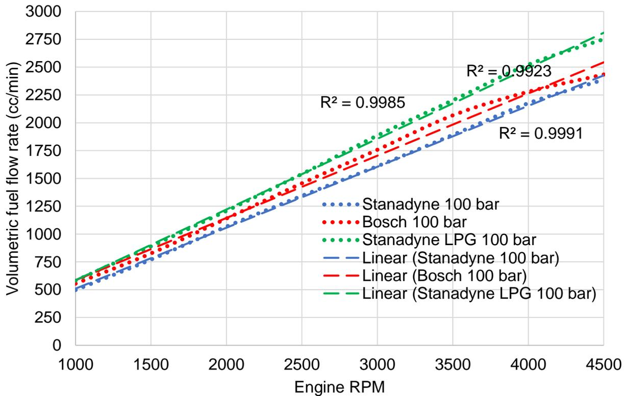
Figure 14: Volumetric fuel flowrate of three DI pumps @100 bar at 30°C fuel temperature.
