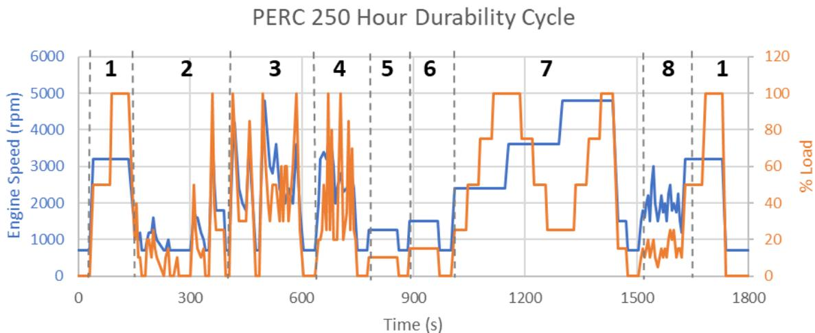
Figure 12: Modes in 30-min Durability cycle designed for 250 hrs. of durability testing.
