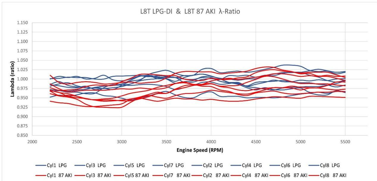
Figure 34: Individual cylinder lambda with respect to speed for both gasoline and LPG baseline testing.
