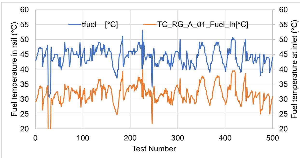
Figure 43: Fuel temperatures in injector rail and pump inlet showing the pump compression effect.
