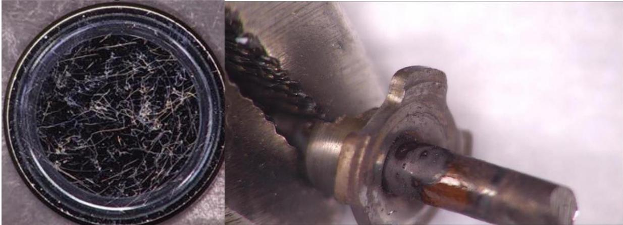
Figure 56: High-side DI pump outlet valve (left) and DI injector retainer and armature interface (right).
