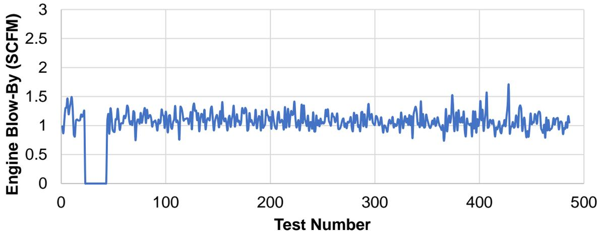
Figure 53: Engine blow-by trend during durability testing.
