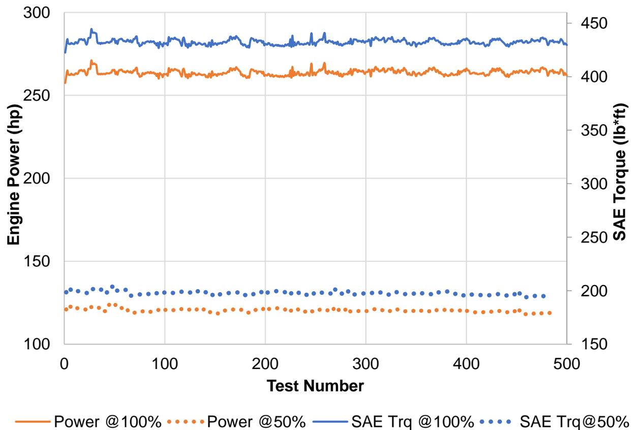
Figure 49: Variation in engine power and torque characteristics during durability testing.
