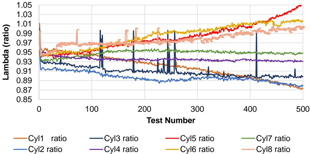
Figure 44: Lambda ratio and its deviations for each engine cylinder
