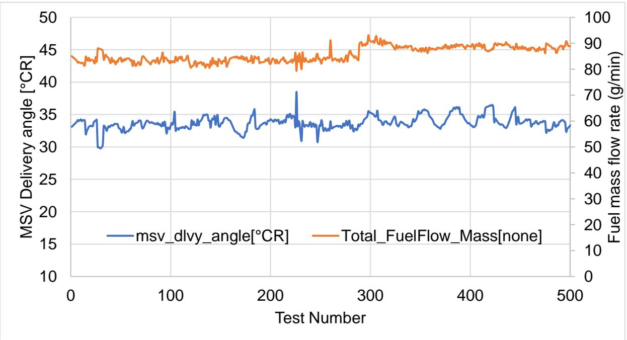
Figure 42: Stable MSV delivery angle and engine fuel mass flow rate of high-side fuel pump at 1250 RPM, 15% load (low throttle & low idle condition).
