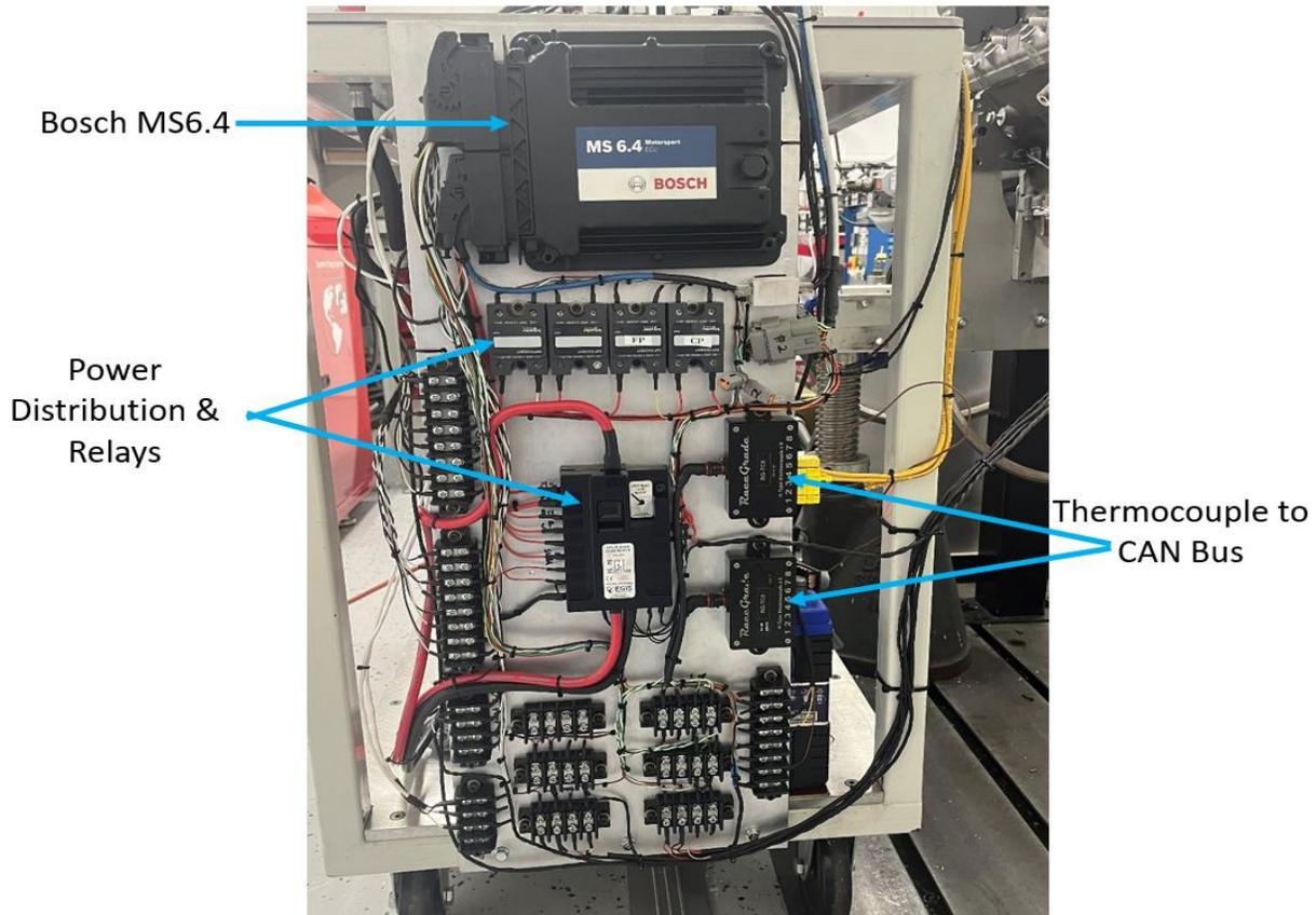
Figure 7: Image of ECU, power distribution relays, and data loggers
