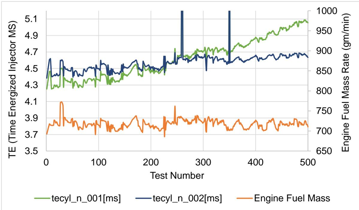
Figure 46: Variation in the injector energization time and engine fuel mass flow
