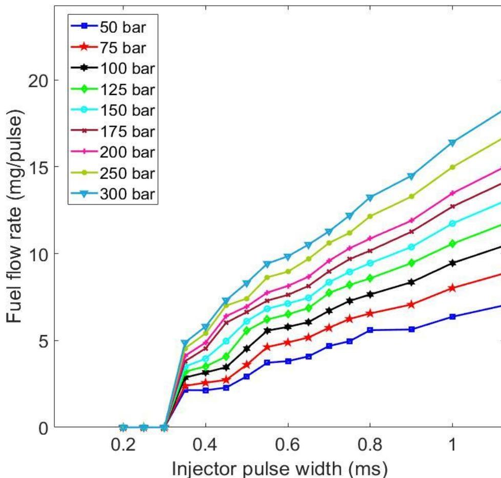
Figure 29: Injector flow rate variation with respect to pulse width
