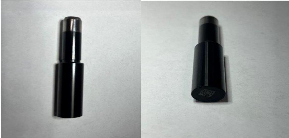
Figure 25: Image of pump pistons after durability testing
