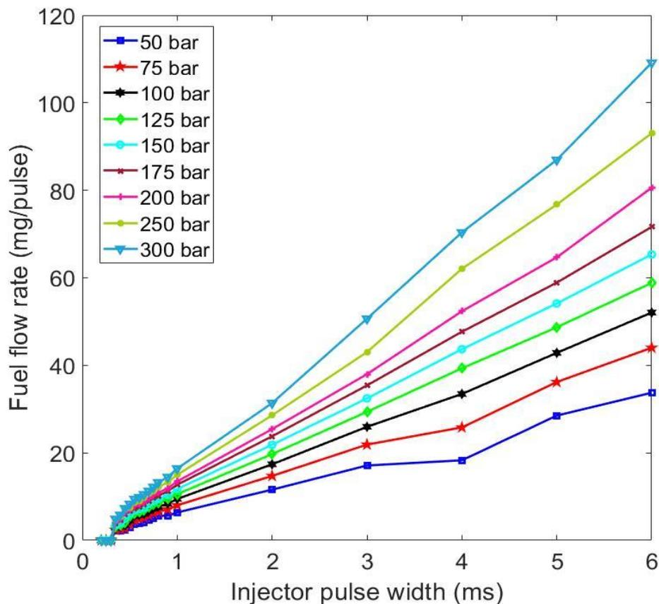
Figure 28: Injector flow rate variation with respect to pulse width (Bosch)
