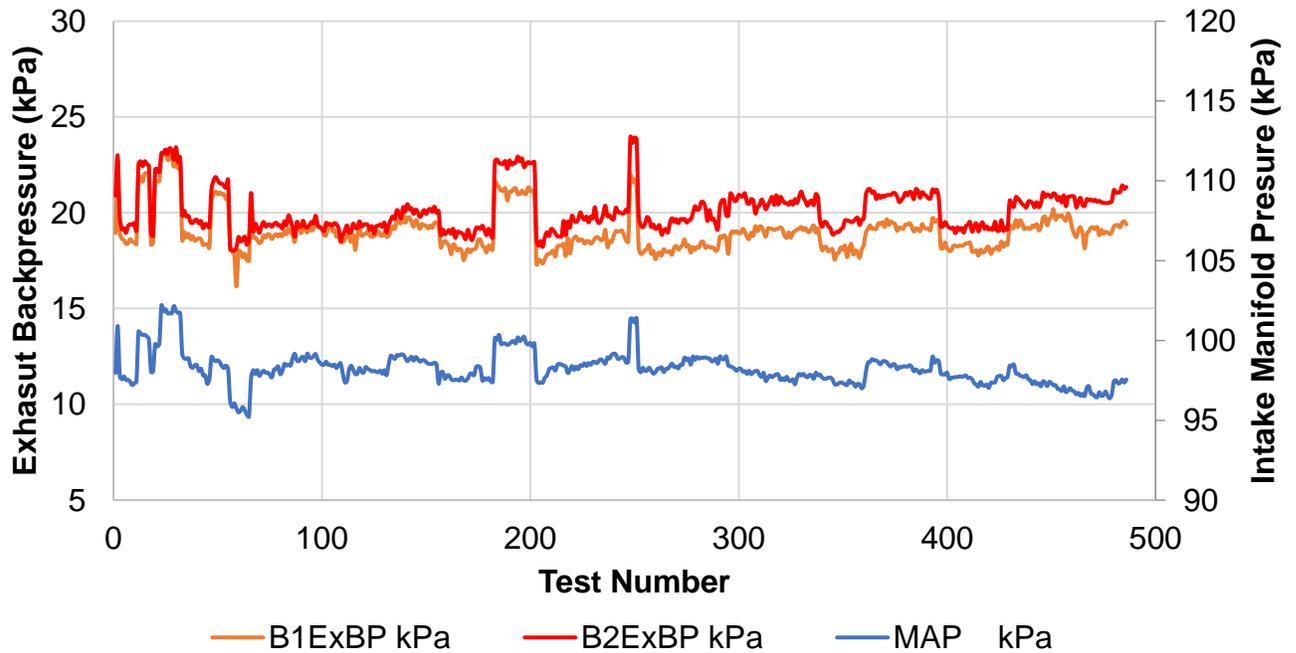
Figure 51: Variation in exhaust back pressures and intake manifold pressures during durability testing.
