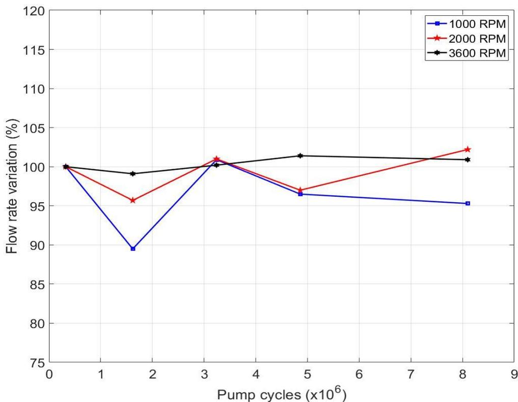
Figure 23: Flow rate variations for Stanadyne 200 pump at three different speeds during the 25-hr. pump reliability testing
