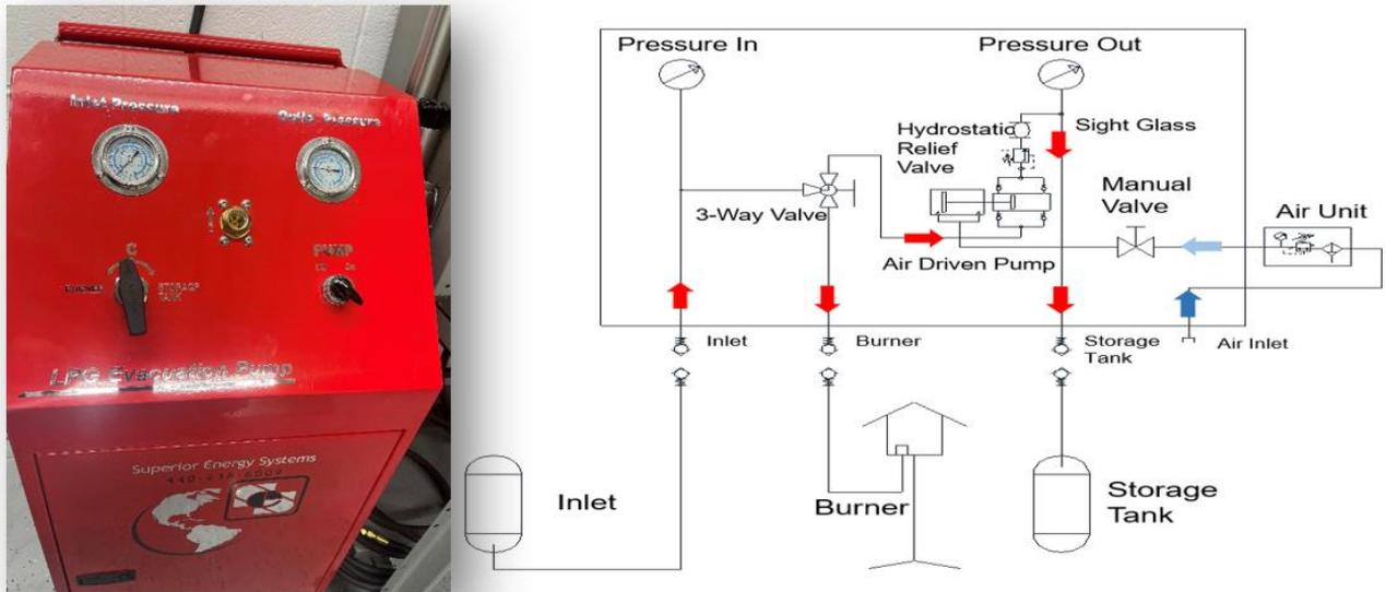
Figure 4: LPG evacuation system & its operating schematic.
