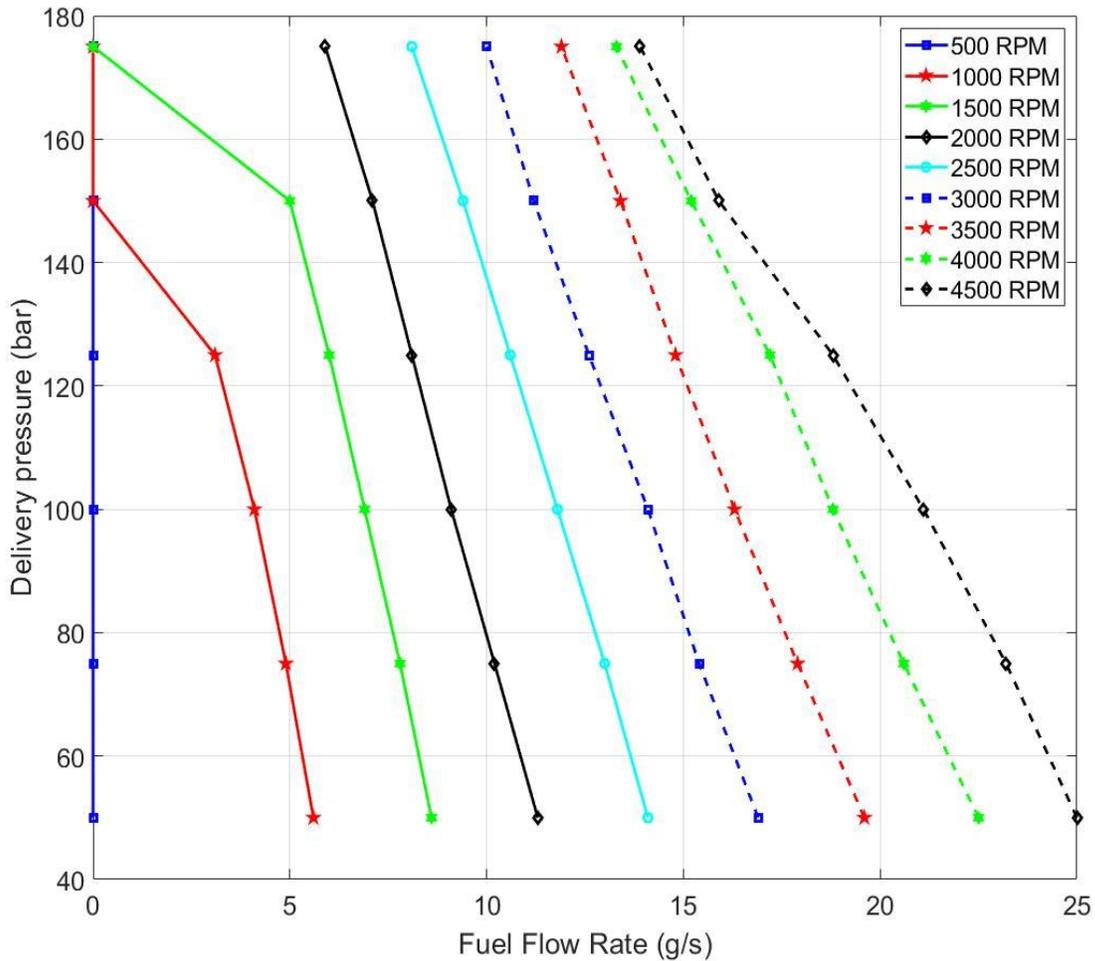
Figure 16: Mass flow rate variation with respect to engine speed and delivery pressure for Stanadyne SP1200 – 200 bar pump.
