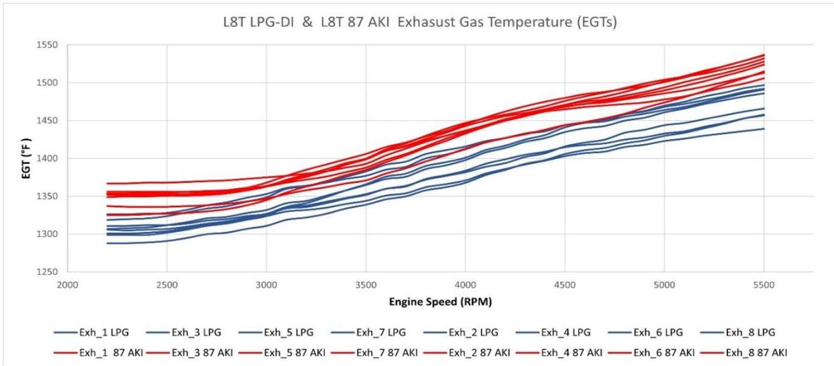
Figure 36: Exhaust gas temperatures of individual cylinders at different speeds with 87AKI gasoline and LPG DI operation
