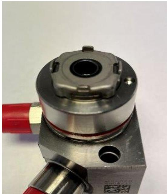
Figure 26: Image of lower pump piston seal of Stanadyne SP1200 – 200 pump
