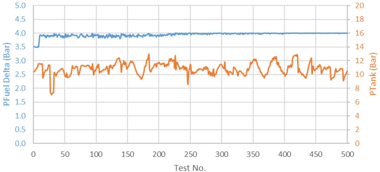
Figure 39: Fuel Delta pressure and Fuel Tank pressure at 3200RPM WOT during 250 hrs. durability testing.
