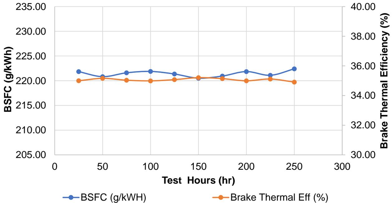
Figure 50: Variation in BSFC and BTE during 250 hrs. of durability testing.
