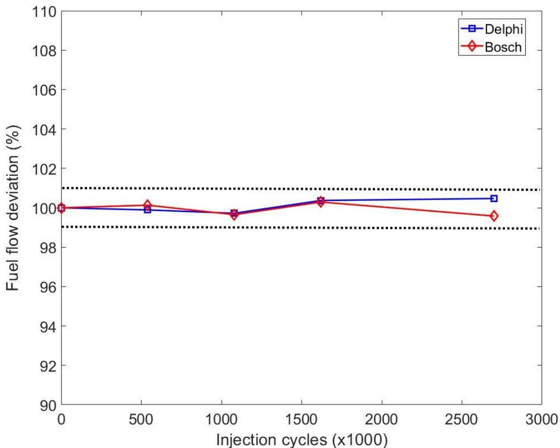
Figure 30: Flow rate deviations of Bosch & Delphi injectors during the 25-hr. injector reliability testing
