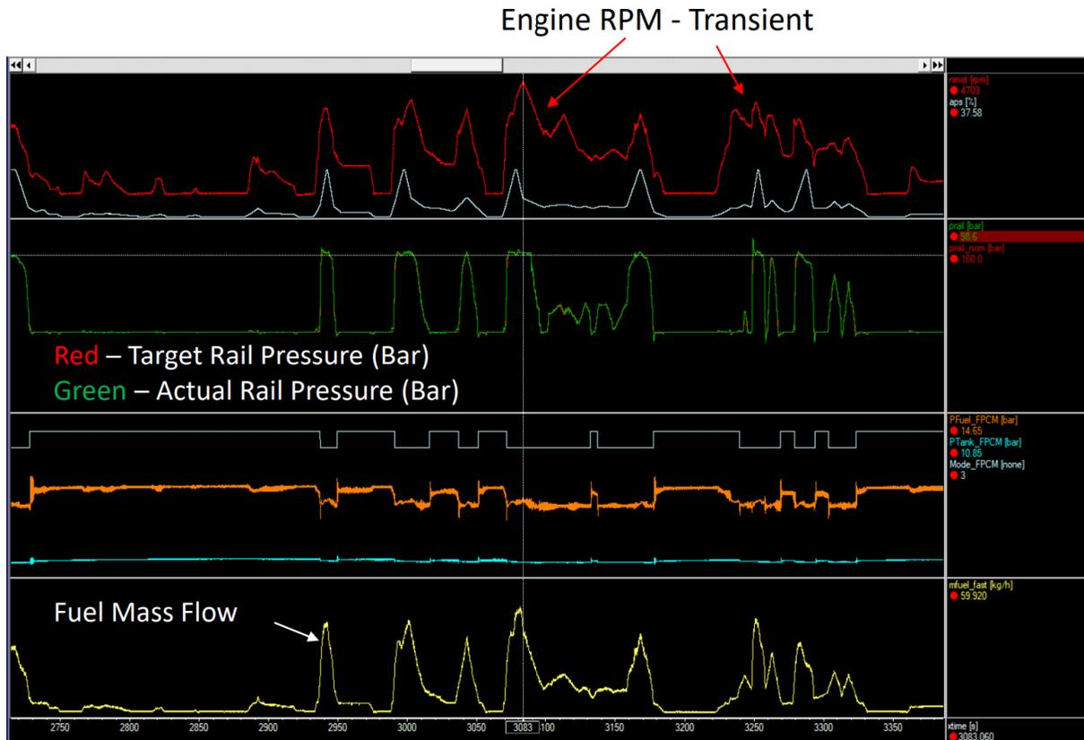
Figure 55: ECU screen depicting various parameters during transient operation.
