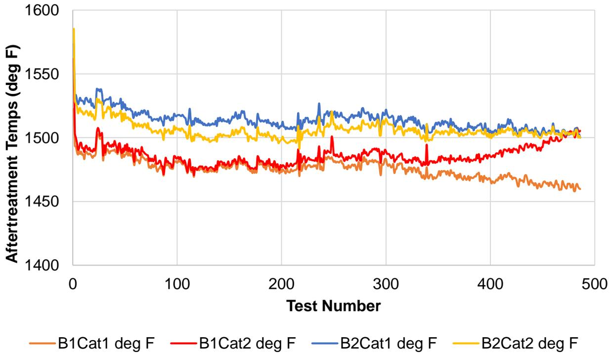
Figure 52: Variation in pre and post catalyst temperatures for cylinder banks 1 and 2.
