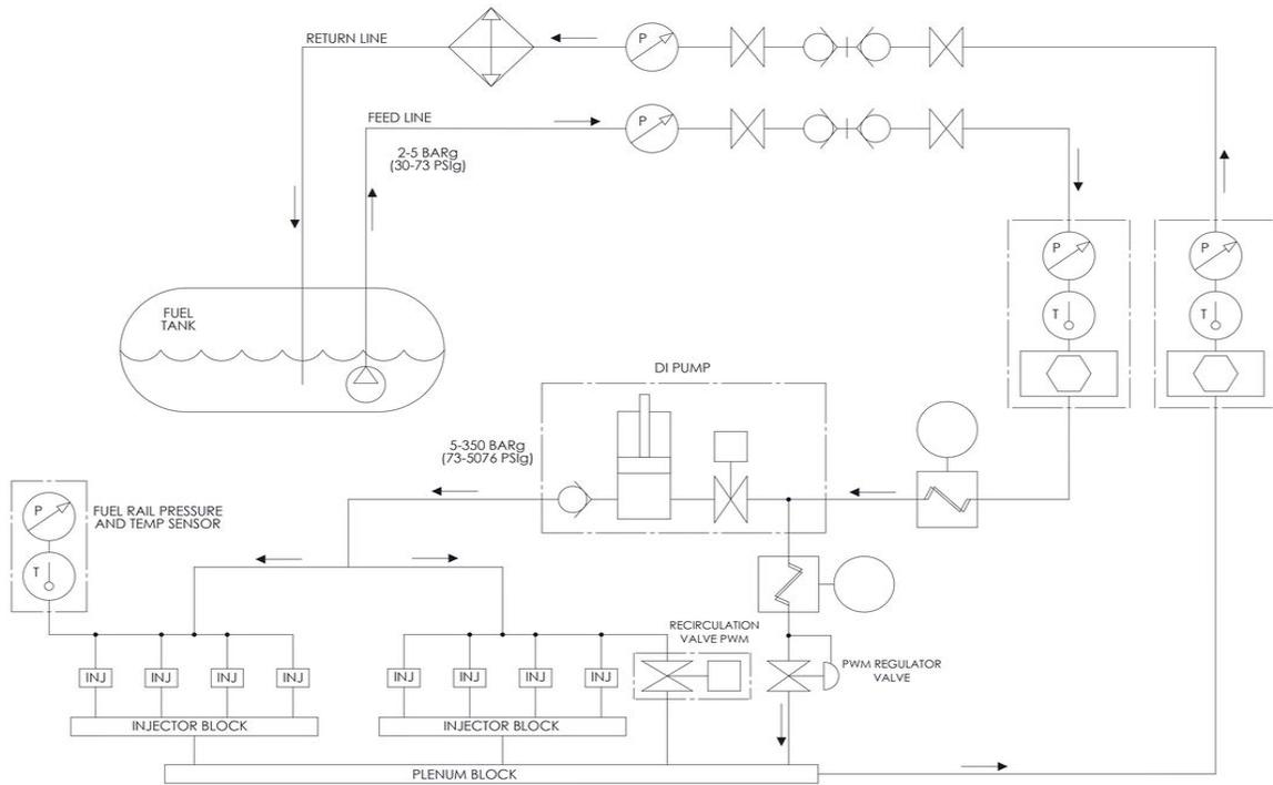
Figure 2: Schematic drawing of the high-pressure DI pump test rig
