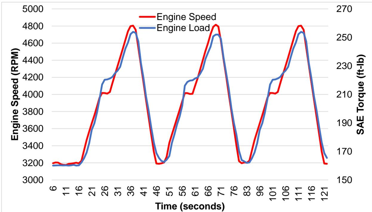
Figure 11: Stage II Engine Break-In procedure during engine shake down process.
