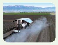
Before planting, the Soil Steamer injects steam along the intended seed rows using continuously moving banded applicators. To lower energy consumption and costs, these applicators are designed for shallow steaming, applying steam to only the necessary area — the top 1–2 inches of soil where weed seeds tend to germinate.
