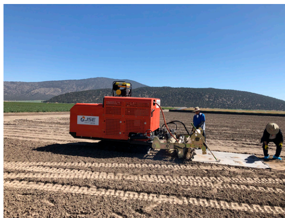
Fig. 2. The Steamy steam applicator from JSE, Republic of Korea, used in spinach trial 3.
