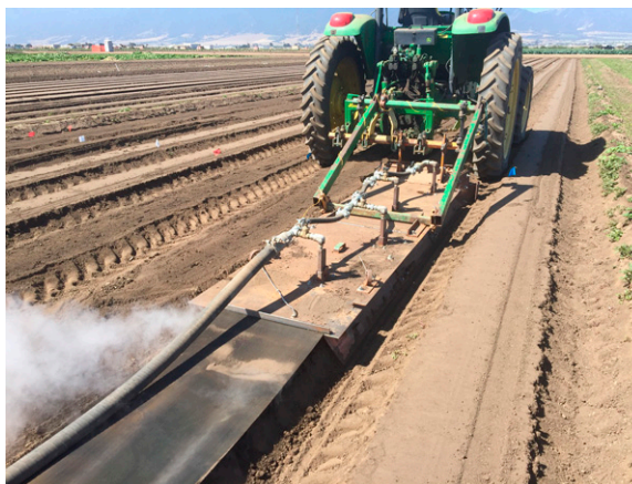
Fig. 1. The fabricated bed shaper used as a steam applicator used in lettuce trials 1 and 2.
