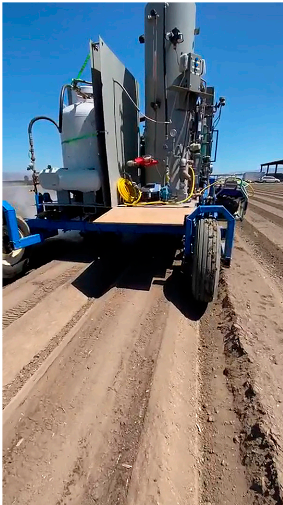
Fig. 3. University of Arizona steam applicator used in carrot trial 5 and lettuce trials 4 and 6.
